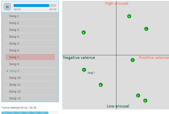
Fig. 1. The graphical interface used in the emotion annotation tasks. The square panel on the right represents the VA plane with valence and arousal as the horizontal and vertical axes, respectively. Upon a subject clicks on the panel and labels the VA value of a song, a green dot showing the song ID is displayed at the specified VA coordinates. The subject can drag and drop the green dots to edit the annotations. The panel on the left shows the song list and provides a playback interface.
